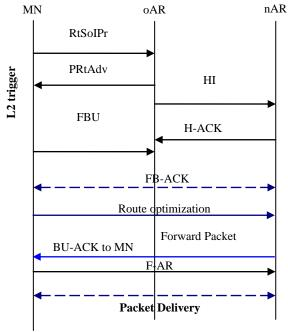
Fig. 1. Message exchange during handover.
