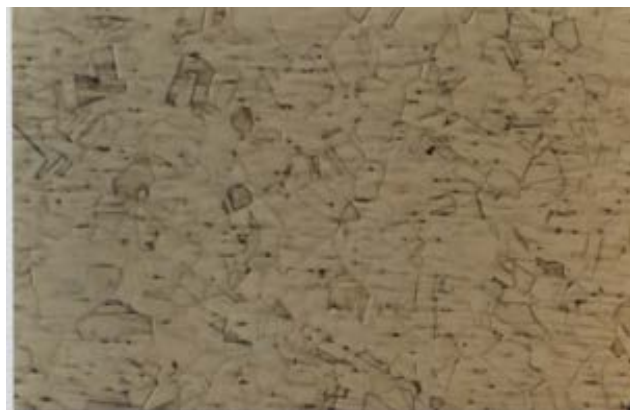
Fig. 1 Microstructure of the base metal as-received after streicher testing – 200X.
