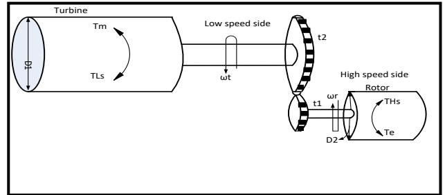
Fig. 3. Wind Turbine Drive Train [15]
