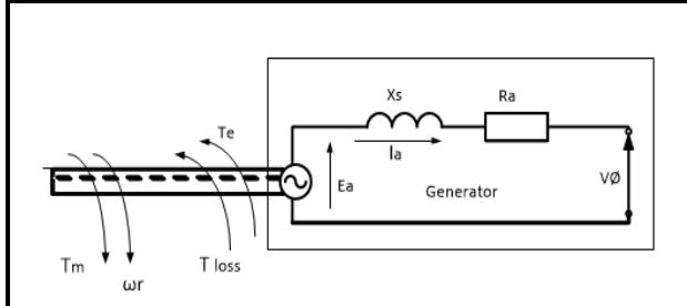
Fig.4. Synchronous machine operated as a generator [8]
